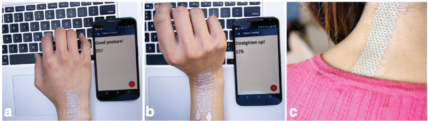
Figure 11. Strain gauge for body position sensing. a) The strain gauge reading indicates that the user's wrist is in a correct typing position. b) The strain gauge reading indicates that the user's wrist is not at a correct posture, which causes the mobile phone to send a warning message. c) The strain gauge can also be worn on other body positions, such as the neck and back, to detect movement and posture.
