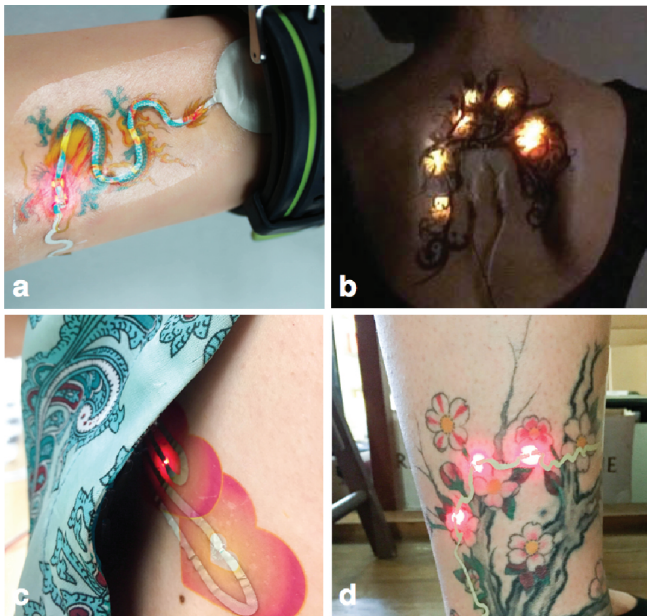
Figure 7. Example of Skintillates tattoo displays. a) a dragon Skintillates display is powered by the watch and could serve as a point-light display, b) a back Skintillates tattoo that flashes with the beat of the music around the wearer, c) a private Skintillates tattoo flashing according to ECG signals, d) a Skintillates tattoo without a printed art layer decorates an existing permanent tattoo
