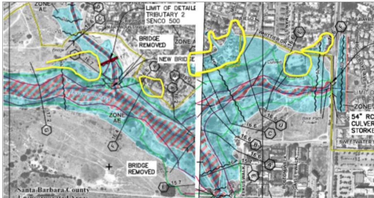
Figure 35. Pre-project flood hazard map that shows the proposed revision as a faint green line and residential areas to be removed from the flood hazard zone with the yellow highlighting.
