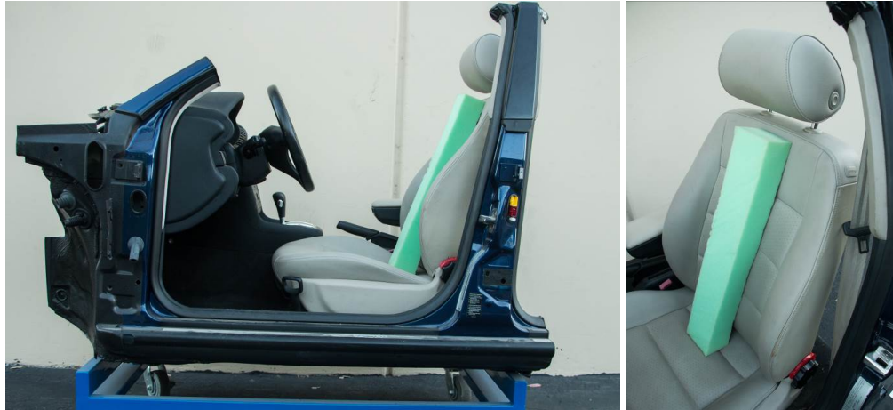
Figure 5: Cut-away driver seat apparatus with soft green foam block attached to the seatback.
