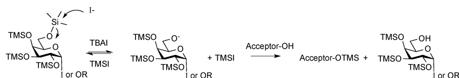
Figure 14. Limiting TBAI to 1.5 equiv minimizes trans-silylation side reactions.
