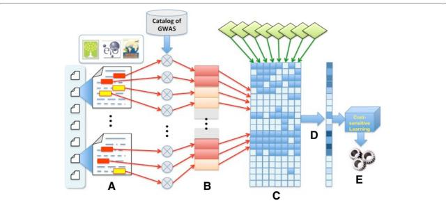
Fig. 3 System architecture. Our proposed system architecture summarizing the steps (a-e) in the machine learning training process
