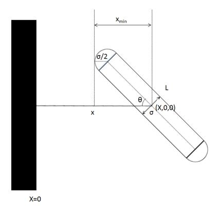
**Figure 5-9** The contact potential  $\beta W\left(x_{\min},\theta\right)$  as a function of angle  $\theta$  between a hard spherocylinder and a flat wall. The length of the hard spherocylinder is  $L=10\sigma$  and the packing fraction for the hard spheres in the bulk is  $\eta=0.2239$ . The solid line is from DFT by R. Roth [170], the dashed line is from AO theory, and symbols represent the MC-DFT results.
