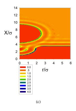
**Figure 5-8** Schematic of a hard rod near a wall (y=0 plane cut) in a hard-sphere solvent. The spherocylinder is placed at (x,0,0) while the wall is at x=0. The closet distance between them is  $x_{\min}(\theta) = (\sigma + L|\cos\theta|)/2$ .
