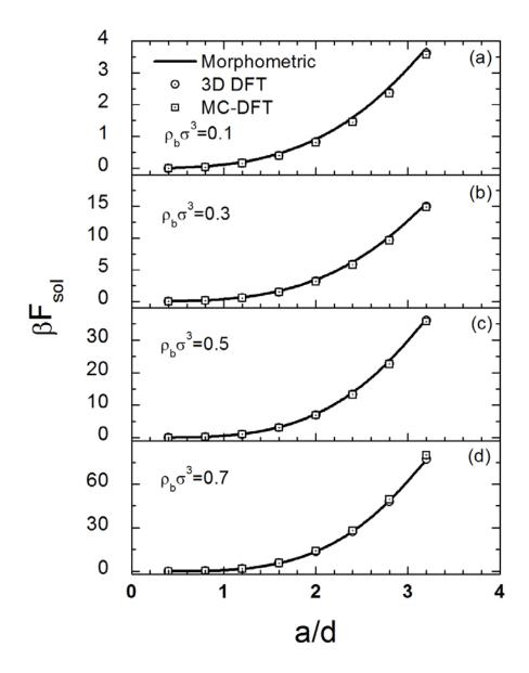
**Figure 9-3** (a) The solvation free energy of a cylindrical **B** of height h = 2d versus radius r in a hard sphere solution with solvent density  $\rho\sigma^3 = 0.1$ . (b) The same as Fig. 9-3(a), except  $\rho\sigma^3 = 0.3$ . (c) The same as Fig. 9-3(a), except  $\rho\sigma^3 = 0.5$ . (d) The same as Fig. 9-3(a), except  $\rho\sigma^3 = 0.7$ .
