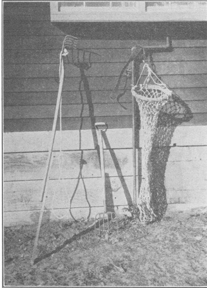
FIG. 1. Gear used in digging Pismo clams. Rake with extension handle and rope by which it is pulled through sand, fork and "drag" with snap and belt
