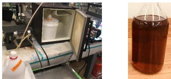
Figure 5. 2 Pre-treatment of fermented food waste feedstock through membrane filtration; left: bench-scale crossflow microfiltration unit; right: fermented food waste permeate after filtration
