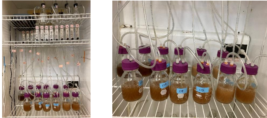
Figure 5. 3 Experimental set-up of bioreactors with forced and humidified aeration
