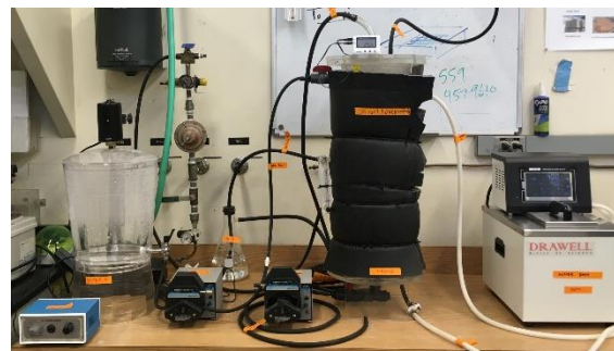
Figure 5. 4 The 6-L benchtop bioreactor system for PHBV production (left: schematic design; right: the actual production system after construction)
