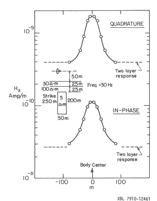
Figure 6. Anomalous electromagnetic response in  $H_x^S$  of a concealed conductor within the second layer of a two-layer earth, calculated at the point of the single coil.
