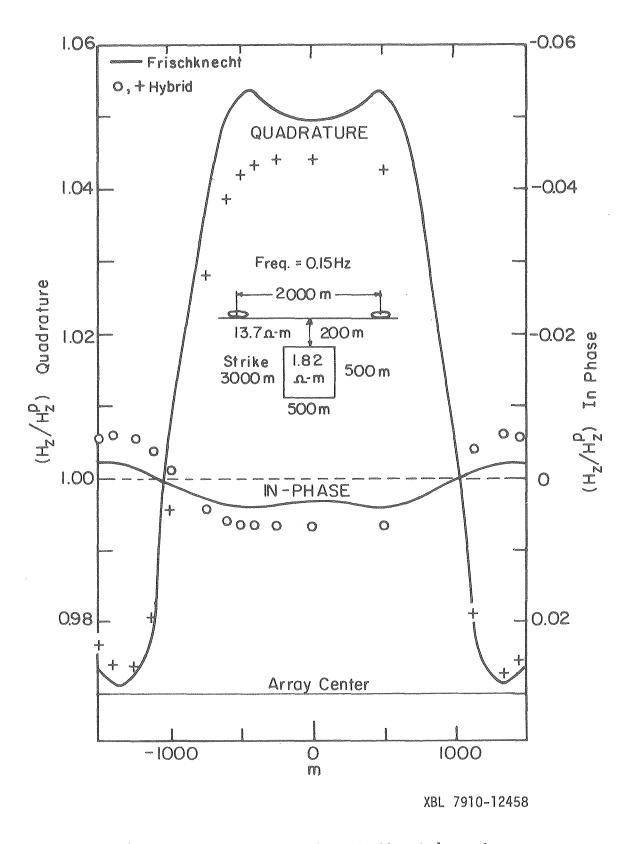
Figure 4. Comparison between the Frischknecht's scale tank model result and the hybrid solution.
