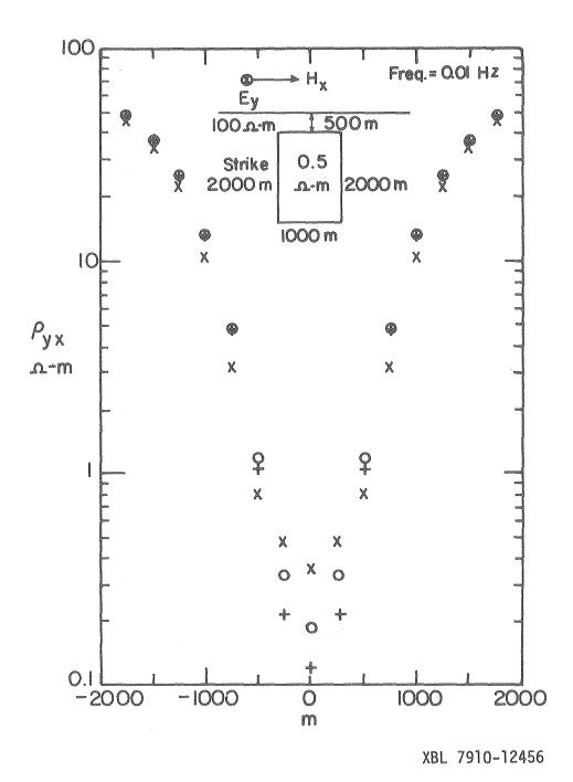
Figure 2. Apparent resistivity,  $\rho_{xy}$ , for the conductive brick model, plotting symbols reference to number of cells used in the calculation, x=40, +=105, 0=168.
