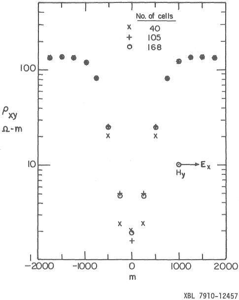
Apparent resistivity,  $\rho_{\boldsymbol{x}\boldsymbol{y}},$  for the conductive brick model. Figure 3.
