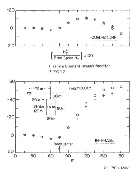
Figure 5. Comparison of the normalized  $H_Z^S$  between the finite element solution and the hybrid solution for a conductive brick; data plotter at the point of the receiver coil.
