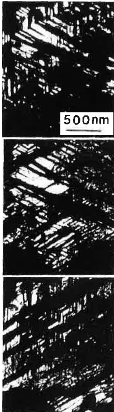
Figure 2.18: Dark field images showing the distribution of the three tetragonal variants in a \sim 6\text{YSZ} material that has been subjected to the c \rightarrow t transformation. Adapted from [77].
