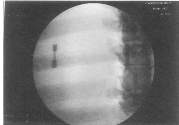
Figure 5. An x-ray image of the chest phantom with the stenosis phantom in place.
