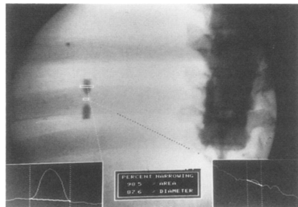
Figure 6. An example of the linear background interpolation method for the measurement of percent stenosis with the chest phantom.
