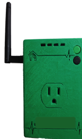
Figure 4.3: IEEE 802.11 connected plug load capable of measuring power information and shedding loads
