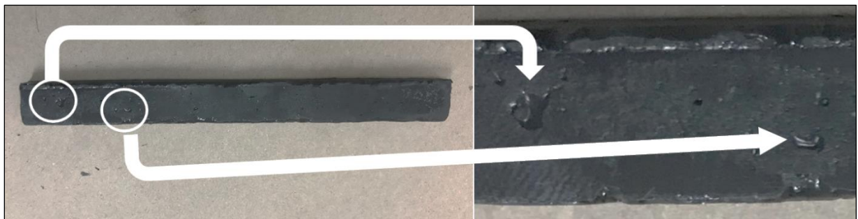
Figure 6.4: Air pockets noted on third replicate specimen.
