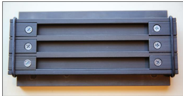
Figure 6.5: Modified mold configuration to produce three beam specimens in a single pour.
