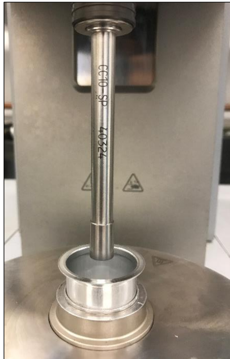
Figure 7.1: Concentric cylinder geometry with 10-mm bob.
