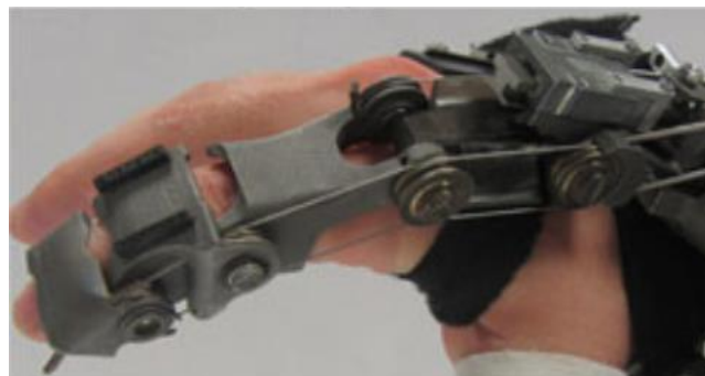
Figure 1.2: HX device with segmented finger interfaces [12].
