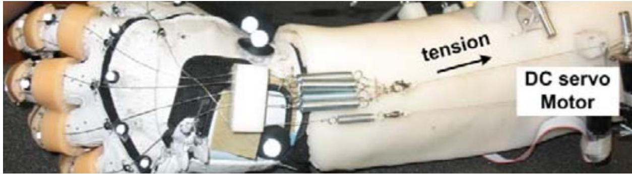
Figure 1.3: BiomHED device with extendon-style passive actuators [13].
