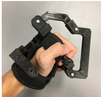
Figure 3.3: Physical prototype of the index finger manipulator with experimentally adjusted link lengths.
