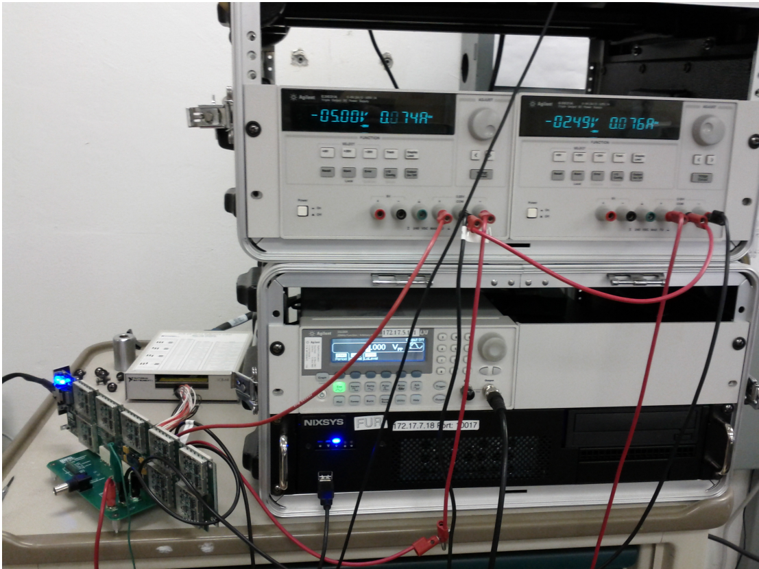
Figure 16.11 – A single AFE17 installed in a test fixture with a rack of support equipment. (from top) Two power supplies provide the four voltages needed for operation, an Arbitrary Waveform Generator (AWG) provides the transmit signal and output amplification, a multi-core computer (equipped with sampling hardware) handles data acquisition, digital processing, and visualization functions.
