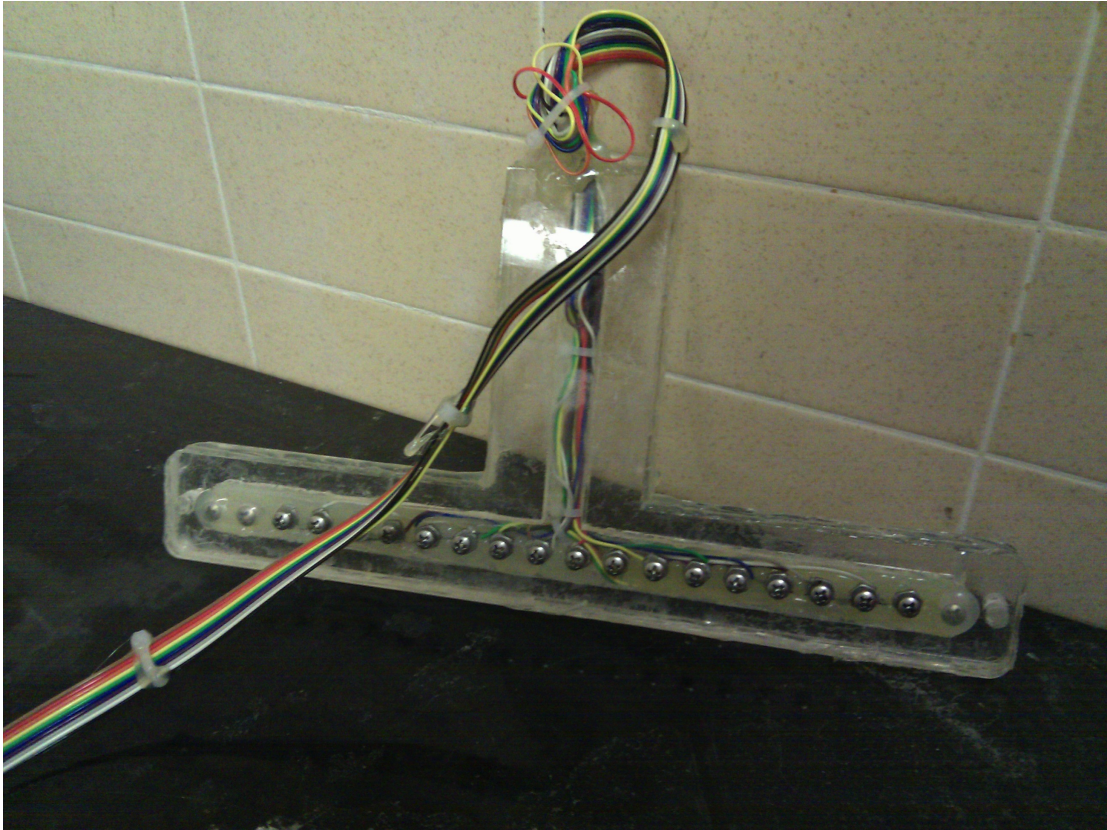
Figure 16.23 – A revised array was constructed making use of stainless-steel 1/4-inch round electrodes to replace the reacting steel of those used with the F68.
