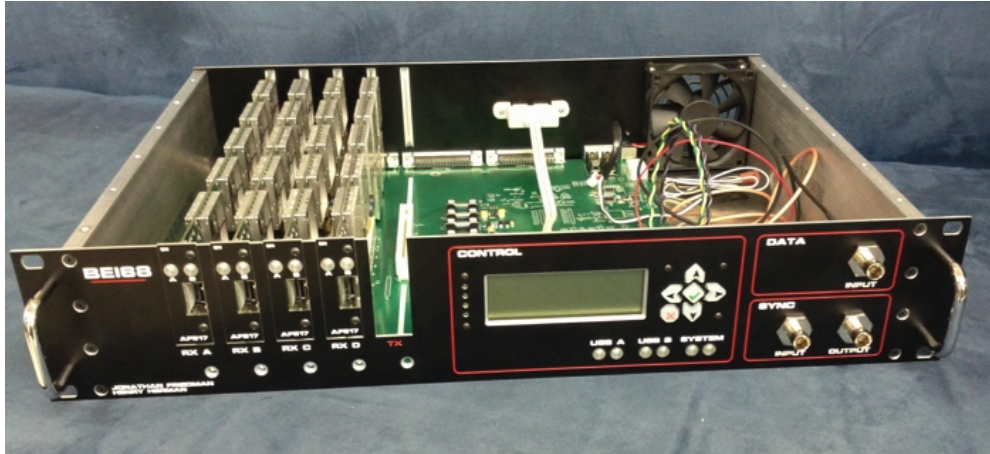
(a) The front of the BEI68 imaging platform. The chassis is two standard rack units in height and can support up to four AFE17 receive cards and one transmit card.
