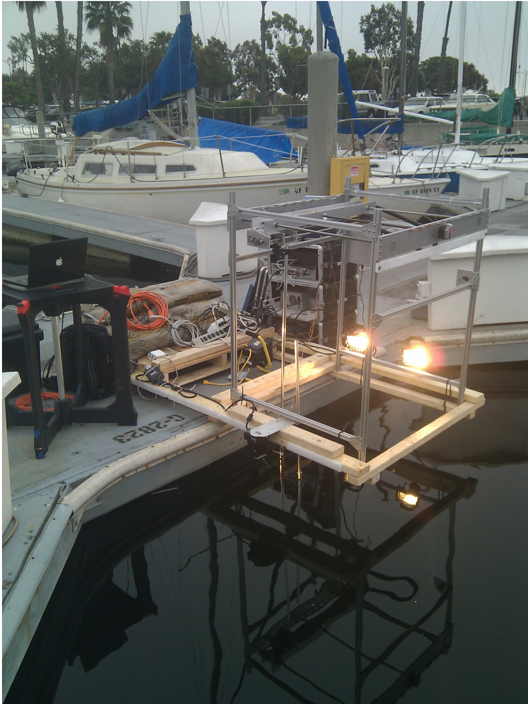
Figure 7.2 – A custom-built motion control platform and cantilever frame was constructed to gather positionally precise high density electric field measurements at depth in the Pacific Ocean.
