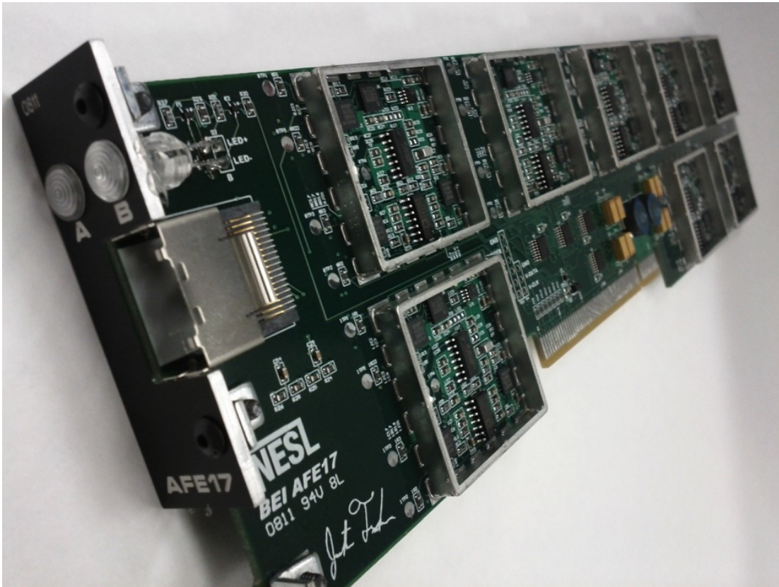
Figure 16.1 – The AFE17 as built. Shown with its shielding covers removed. Each of the square areas contain a complete analog front end. In the distance, near the edge connector fingers, the large power filtering components are visible.
