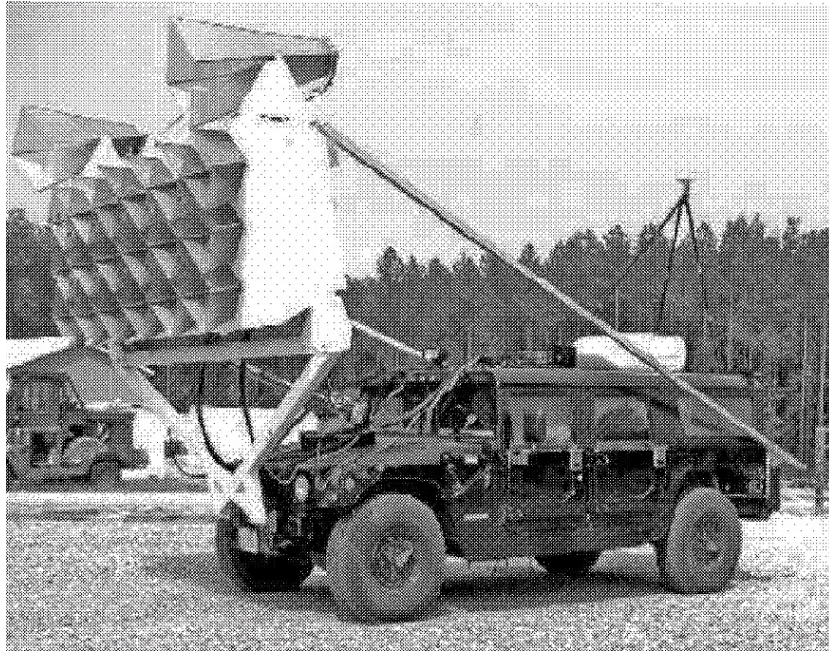
Figure 12.6 – Stanford Research Institute’s forward looking ground penetrating radar system prototype (Reproduced from [SL05]) for near real-time detection of surface emplaced or buried anti-tank mines. This prototype was an outgrowth of military interest which began with [Cor01].
