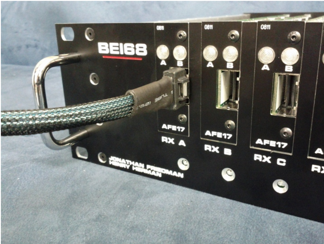
Figure 17.3 – The electrodes attach to the analog processing cards (AFE17's) via a commodity 36-pin mini-SAS connector.
