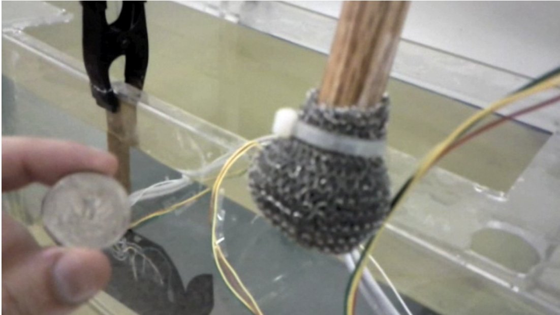
Figure 17.11 – The reference target is a metal sponge coerced into a spherical shape roughly 3.8 cm (1.5”) in diameter. Shown with a U.S. Quarter Dollar.
