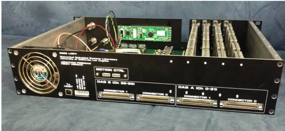
(b) The back panel of the BEI68. ( from left ) The fan exhaust port, the USB interface to the host computer for configuration commands and control feedback, the power input port, ( above ) additional USB peripheral ports for attaching motion control platforms, ( below ) the four shielded mixed signal connectors that interface with the data acquisition cards in the host.
