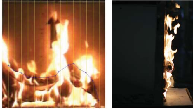
Figure 10: Left : Front video footage during a representative test. The blue contour across the width indicates the measured height of the pyrolysis region. Image taken from the side of a sample during a representative test. Curling of the front layer of cardboard is visible in both images, but the extent of three-dimensional effects is more clearly seen in the side image.
