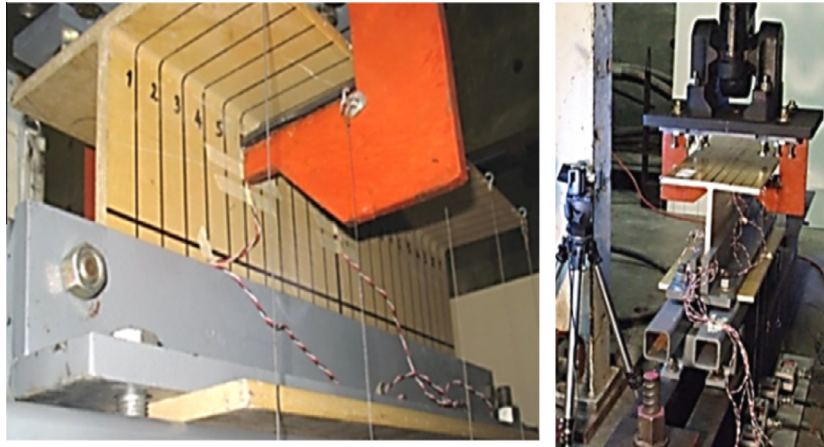
Fig. 6. Typical pull-out web/flange test setup.
