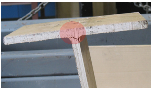
Fig. 37. Failure of 10'' \times 10'' \times 1/2'' (254.0 mm \times 254.0 mm \times 12.7 mm) H-profile.
