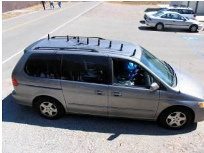
Figure 27: Antenna placement with 8 active OBUs on one vehicle
