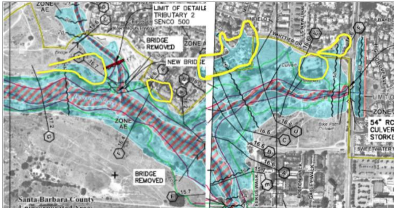
Figure 32. Pre-project flood hazard map that shows the proposed revision as a faint green line and residential areas to be removed from the flood hazard zone with the yellow highlighting.
