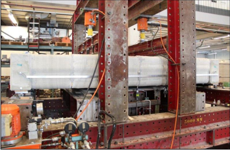
Figure 2.11: Scale-down model tested in a 4-point bending protocol [17].
