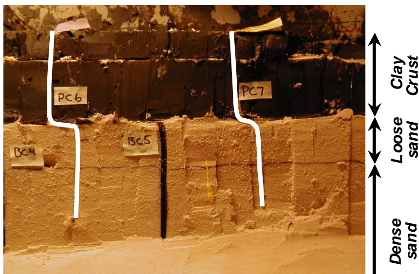
Figure 2-13: Excavation of SJB02 showing the strong localized deformation at the interface between the loose sand and overlying clay layer (paper markers highlighted in white for clarity).
