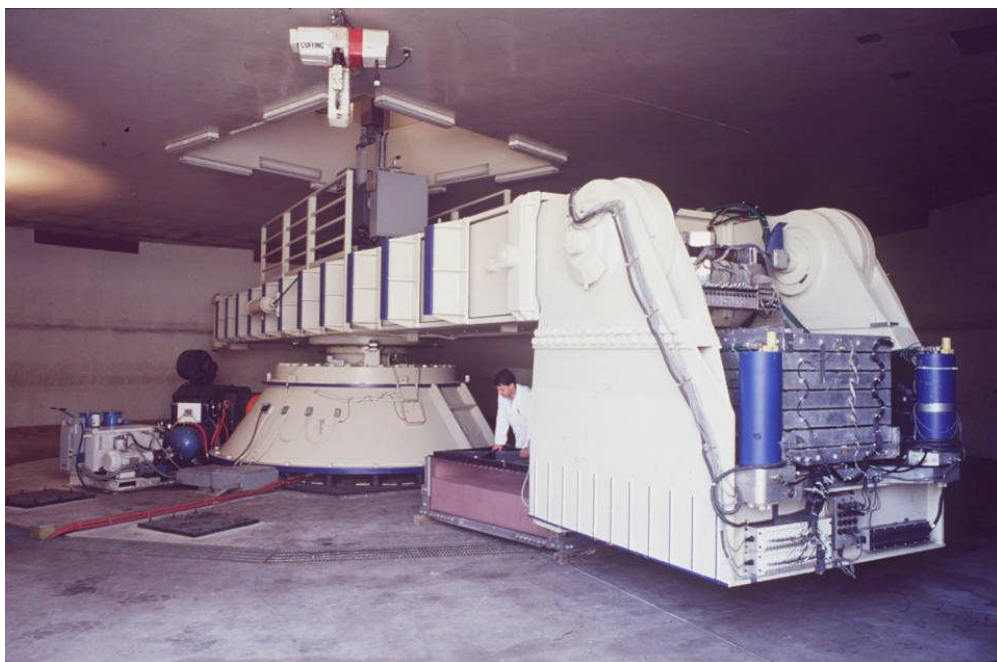
Figure 2-1: 9-m radius centrifuge at the center for geotechnical modeling.
