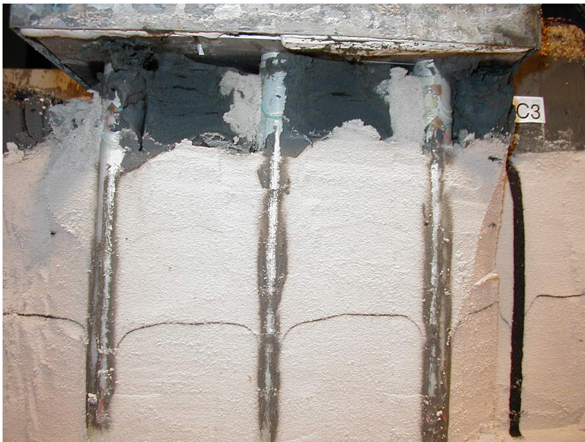
Figure 4-2: Six-pile group from test SJB03 during excavation after shaking.
