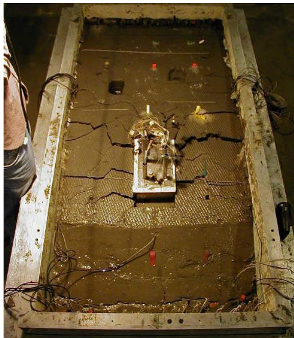
Figure 2-12: Photo of model SJB01 off of the centrifuge after testing with external instrumentation and wiring removed, showing the ground's cracking pattern from spreading toward the open channel (bottom of photo).
