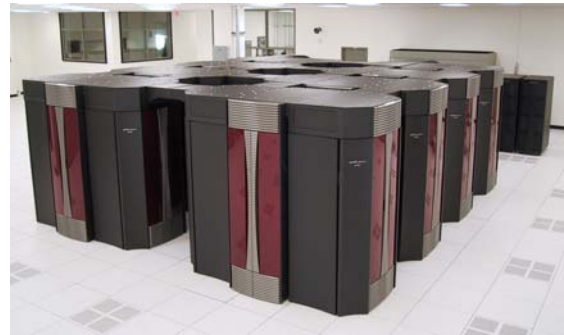
Figure 3: Elevated view of 256-MSP, 8-cabinet Cray X1 at ORNL's Center for Computational Sciences.
