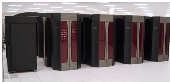
Figure 1: Front view of 256-MSP, 8-cabinet Cray X1 at ORNL's Center for Computational Sciences.
