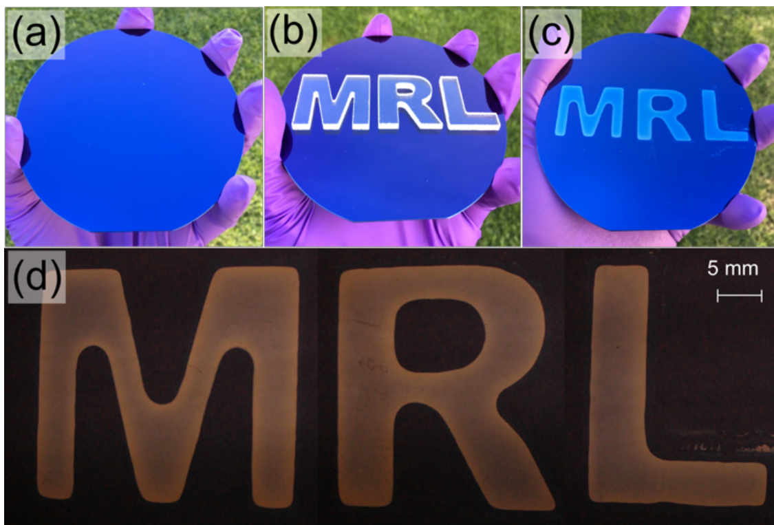
Figure 3. Patterning using glass cover slips of different shape. Digital images showing the preparation of “MRL” brushes on a 4-inch diameter ATRP-initiator functionalized silicon wafer (a) Initiator-functionalized silicon wafer, (b) “MRL” shaped glass cover slips on the wafer prior to brush growth, (c) Resulting polymer brushes after removal of cover slips and extensive washing and (d) Digital micrograph of purified polymer brushes illustrating fidelity with “MRL” shaped cover slips.
