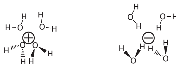
Figure 5-9: Schematic drawing of molecules of water with the negative ends of their dipoles directed toward a cation and the positive ends of their dipoles directed toward an anion.
