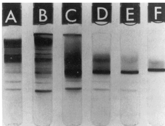
Figure 1-19: Disc electrophoresis on gels of polyacrylamide of native proteins from successive steps in the purification of [acyl-carrier-protein] S-malonyltransferase from E. coli . 190 Electrophoresis was performed on polyacrylamide gels cast from 15% solutions of acrylamide in a discontinuous system of tris(hydroxymethyl)methylamine and glycylglycine. The different gels represent samples from successive steps in a complete purification of the enzyme, seen in its final purified state on gel F. The gels were stained for protein with Coomassie brilliant blue. Reprinted with permission from ref 190. Copyright 1973 Journal of Biological Chemistry .
