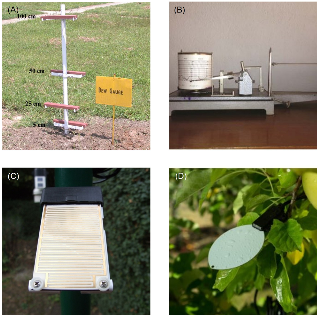
Figure 2.1. (a) Duvdevani dew gauge, (b) De Wit leaf wetness recorder, (c) Davis Instruments resistive leaf wetness sensor, (d) METER Group Phytos 31
