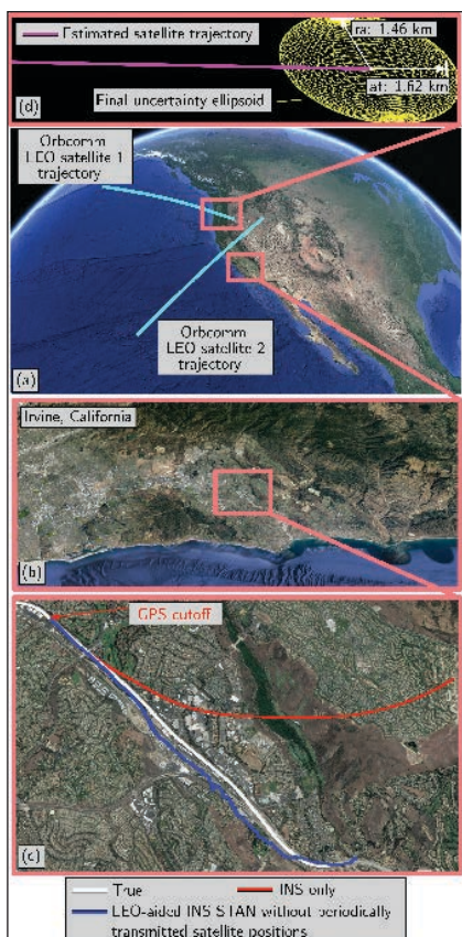
FIGURE 21 Results of the ground vehicle experiment. (a) Orbcomm satellite trajectories. (b)-(c) Ground vehicle true and estimated trajectories. (d) Estimated trajectory and the final 95-th percentile uncertainty ellipsoid for one of the Orbcomm satellites. Map data: Google Earth.
