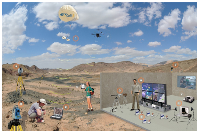
Fig. 1. A model of the different components that are a part of our field recording methodology. A. LiDAR Scanner B. Total Station C. Aerial photography platform D. Digital Note taking (OpenDig) E. Control for Aerial photography platform F. Octocopter forensic imaging platform G. XRF H. Nexcave portable display I. Nextengine 3D scanners J. dGPS K. FTiR L. Digital object photography.
