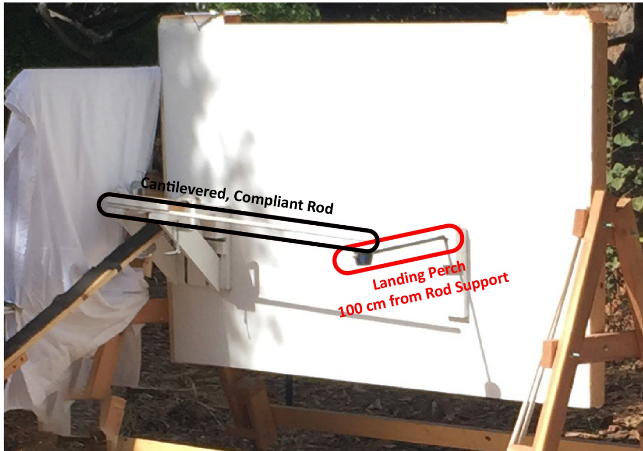
Figure 5.2: Photograph of the wall, branch and perch set up in the field. The rod is cantilevered 90 cm beyond its support. The landing perch is positioned 100 cm from the rod support.
