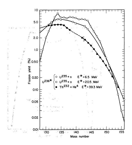
Fig. 19. Heavy wing of the yield-mass curve for U<sup>235</sup>+ thermal neutrons (reference 24), U<sup>235</sup>+ 14-MeV neutrons (reference 25), and Th<sup>232</sup>+ 44-MeV He<sup>4</sup>. The error bar shown indicates the uncertainty in the normalization of the rare-earth relative yields to the Xe relative yields.
