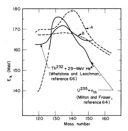
Fig. 13. The average total kinetic energy as a function of the heavy-fragment mass. Curve (A) is calculated from Cameron, so masses and curve (B) from Green's masses for Th<sup>232</sup> (44-MeV He<sup>4</sup>,F).
