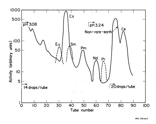
Fig. 1. Elution curve for the light rare-earth elements. Dashed curves represent interpolated positions from rare-earth systematics and column calibration.
