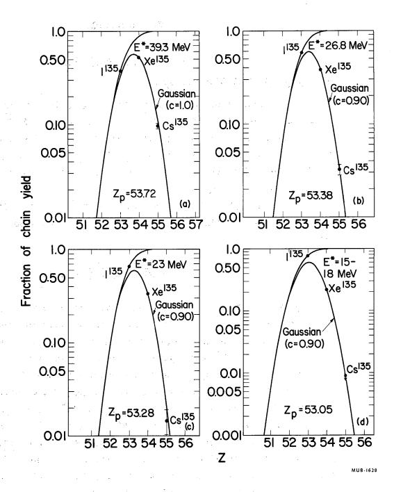
Fig. 5. Gaussian charge-distribution curves fitted to fractionalyield data. The iodine fractional cumulative yields are fitted to an integrated curve based on the Gaussian distribution.
