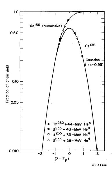
Fig. 7. Fractional yields of  $Xe^{136}$  and  $Cs^{136}$  as a function of  $(Z-Z_p)$ . The  $Xe^{136}$  cumulative yield is based on the mass-136 chain yield obtained from an extrapolation of lighter-mass Xe chain yields. The  $Cs^{136}$  fractional yields for  $U^{235}(He^4,F)$  are those of reference 58.
