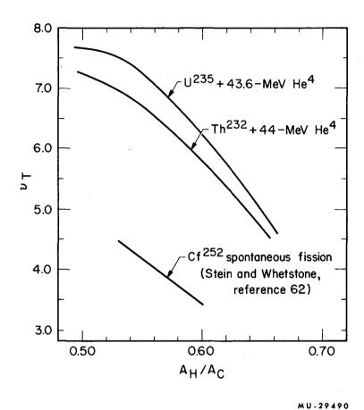
Fig. 12. Total number of neutrons emitted per fission vs the mass fraction  ${\rm A_H/A_C}$ ;  ${\rm A_H}$  is product mass after neutron emission.
