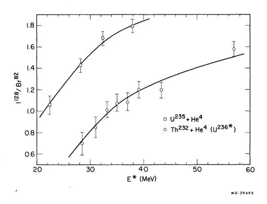
Fig. 10. Fractional chain yield of  $I^{128}$  relative to the Br $^{82}$  fractional chain yield as a function of excitation energy for  $Th^{232}(He^4,F)$  and  $U^{235}(He^4,F)$ .
