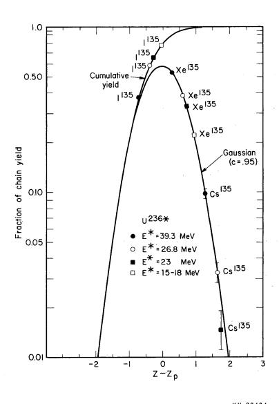
Fig. 6. Gaussian charge-distribution curve which best fit the fractional yield data of the mass-135 chain for all energies.
