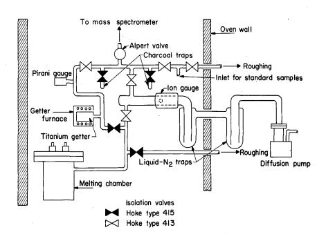
Fig. 3. Schematic diagram of the rare-gas handling and purification system.
