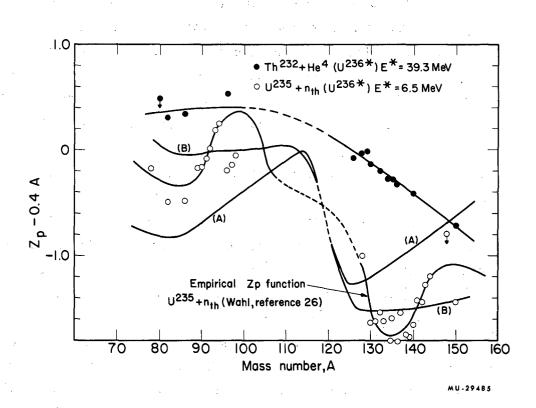
Fig. 16. The empirical Z 's for  $U^{236*}$  are compared; and the comparison of empirical  $Z_p$ 's for  $U^{235}(n_{\rm th},F)$  with those predicted by UCD curve (A) and MPE curve (B) are made.
