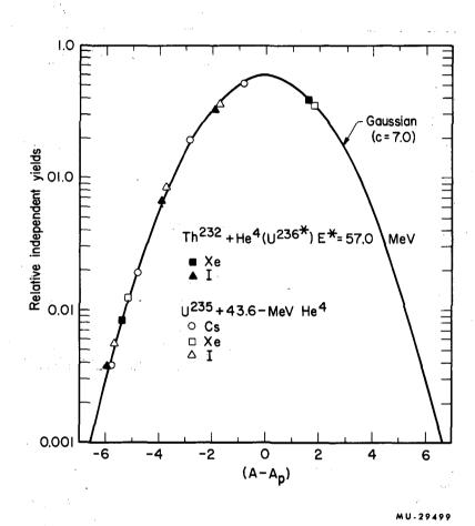
Fig. 20. Relative independent yields of I, Xe, and Cs isotopes vs mass number,  $(A-A_p)$ .
