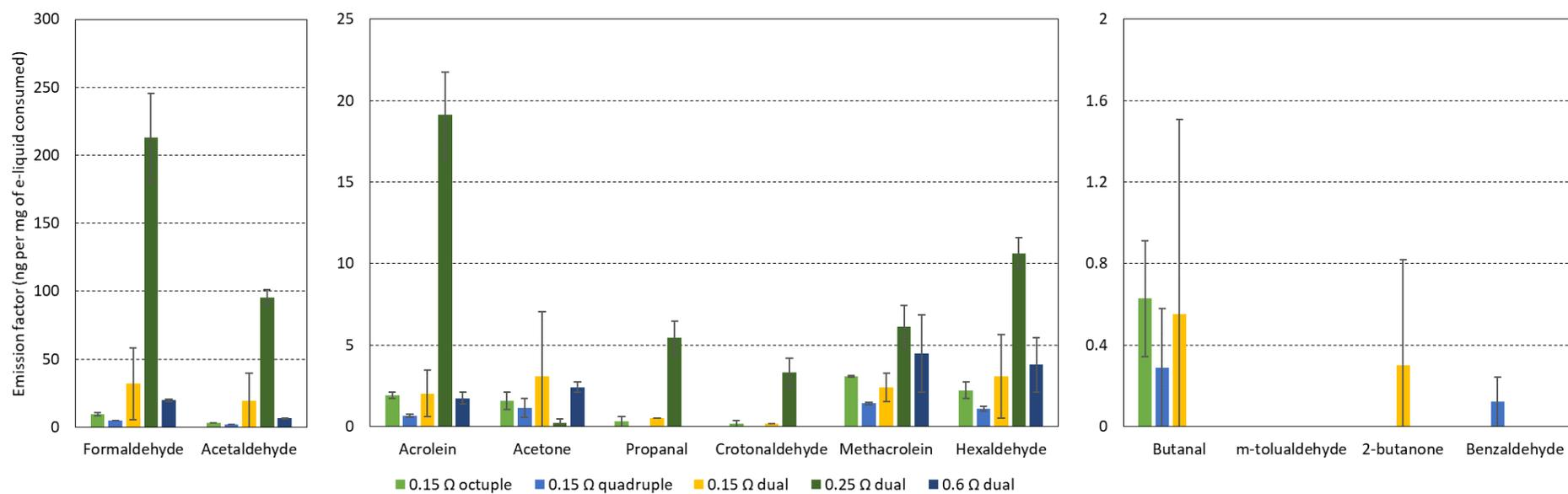
**Figure 5.** Emission factors for volatile carbonyls (puff volume = 50 mL, 50% airflow system vents open).
