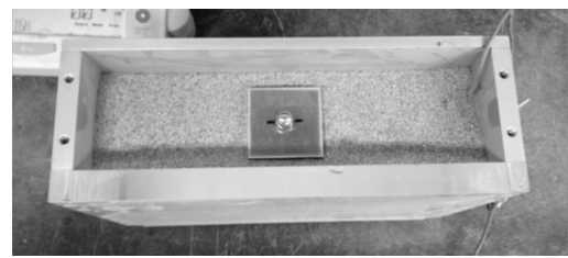
Figure 7. Top of sand layer with square footing
