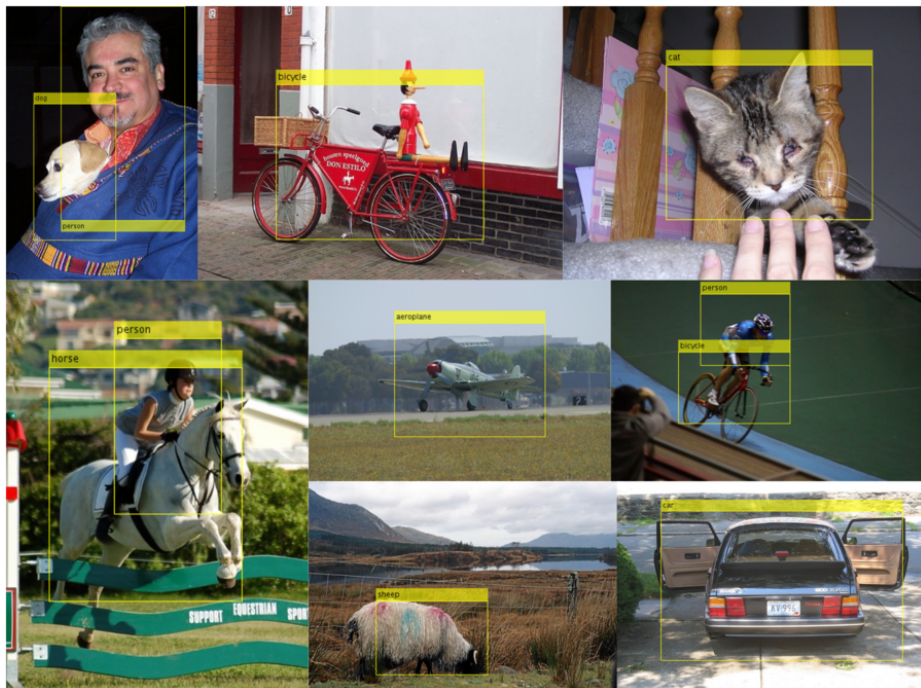
Fig. 6. Visual sample results from the proposed method for Pascal VOC 2007 test set. Yellow rectangles overlaid on the images represent location and extent predictions. The locations of objects in the shown images are accurately estimated. Considering that only image-level labels are used for training, extent estimations are a challenging problem in this setting.
