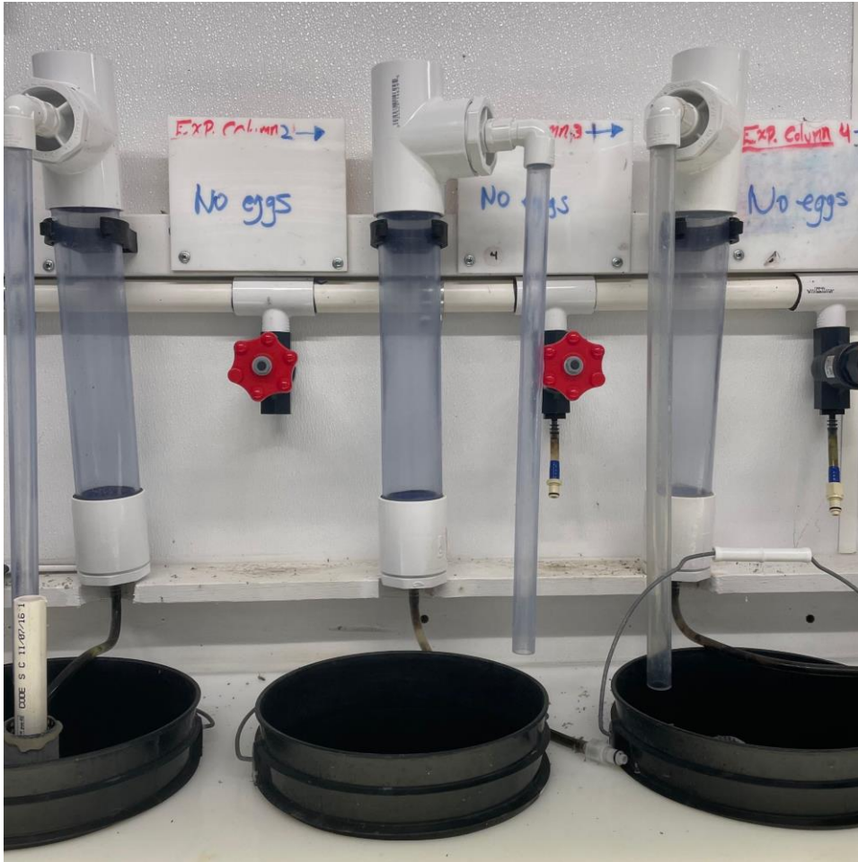
Figure 2.3 Incubation columns in the Egg and Live Prey Production Room at the FCCL. These columns are specifically designed for the incubation of Smelt eggs. During operation, fine sand fills the columns and water flows from the base of the columns, with the flow rate being controlled and modulated by the red valves as shown. This regulated water flow induces a gentle tumbling action for the eggs, which minimizes the likelihood of fungal contamination.
