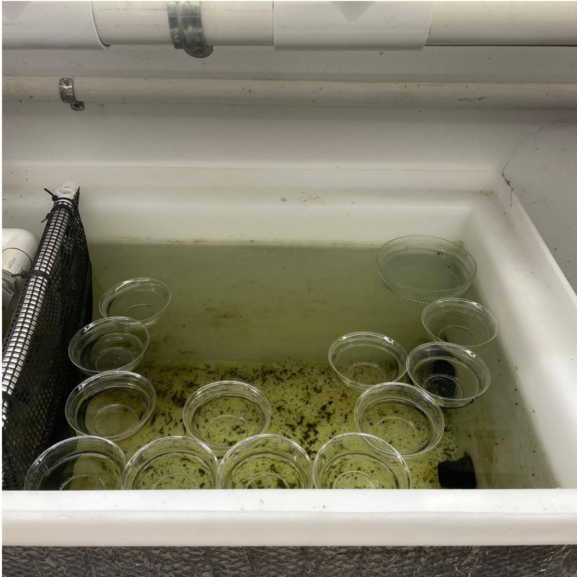
Figure 3.3 The sump of the Delta Smelt incubation system. To maintain a constant temperature, water circulates within the system and the water temperature is regulated by a water chiller. The water within these bowls is refreshed every 24 hours using water from the sump.
