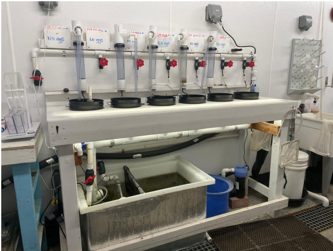
Figure 2.2 An egg incubation system at the FCCL. The system consists of upper incubation columns filled with fine sand, middle black buckets, and a water reservoir. Water is pumped from the reservoir to the columns, where regulated flow agitates the sand, ensuring fish egg movement and reducing fungal growth. As eggs hatch, larvae move to the buckets before water returns to the reservoir, creating continuous circulation. The water was maintained at 16.5°C for Delta Smelt and 12°C for Longfin Smelt.
