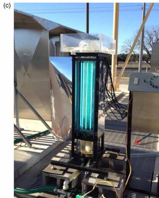
Figure 1 | (a) Three-dimensional rendering of the UV system, (b) schematic giving system dimensions, (c) photograph of system in operation.
