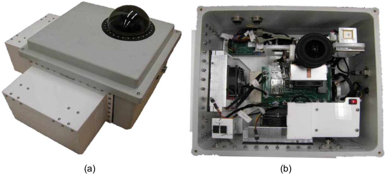
Figure 1: The University of California, San Diego Sky Imager (USI). (a) Outer view showing the enclosure with dome and white radiation shields for the coolers; (b) a top view of the open system showing the components inside the enclosure.
