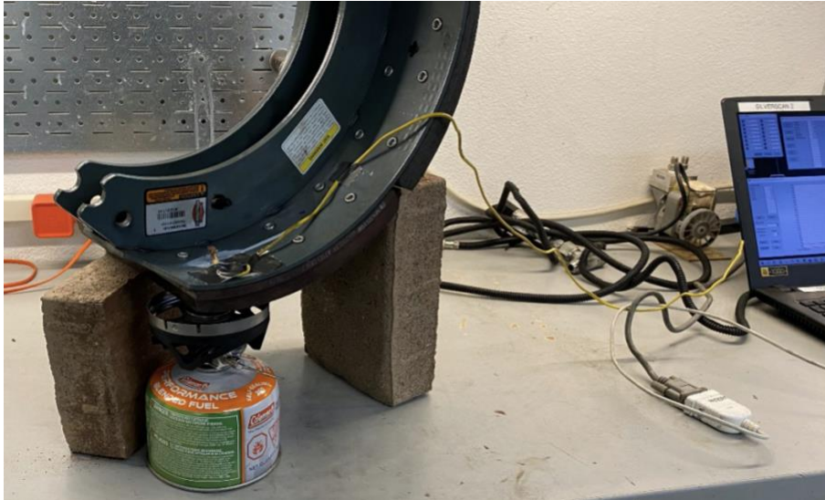
Figure 32. Brake setup with blue flame heat source. Note: The butane camping stove was setup to produce a 3" diameter blue flame ~1" from the surface. Data was logged with a CR10x data logger.
