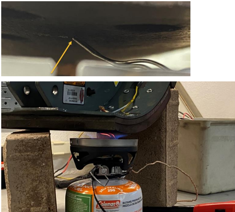
Figure 33. Measurement of the brake pad surface temperature for consistent heat input. Note: This figure shows the detail of the exposed tip forced up against the brake in the top picture and glowing red in the lower picture.
