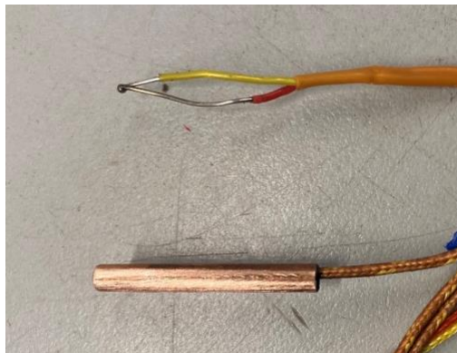
Figure 35. Probe tips: brake test probe (bottom) used in the study and exposed tip (top).
