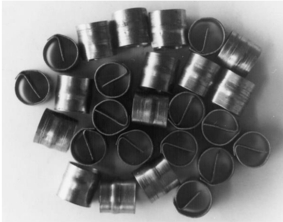
Fig. 1.7. Leasing ring used by Valraj et al. to improve thermal conductivity of Paraffin [42].
