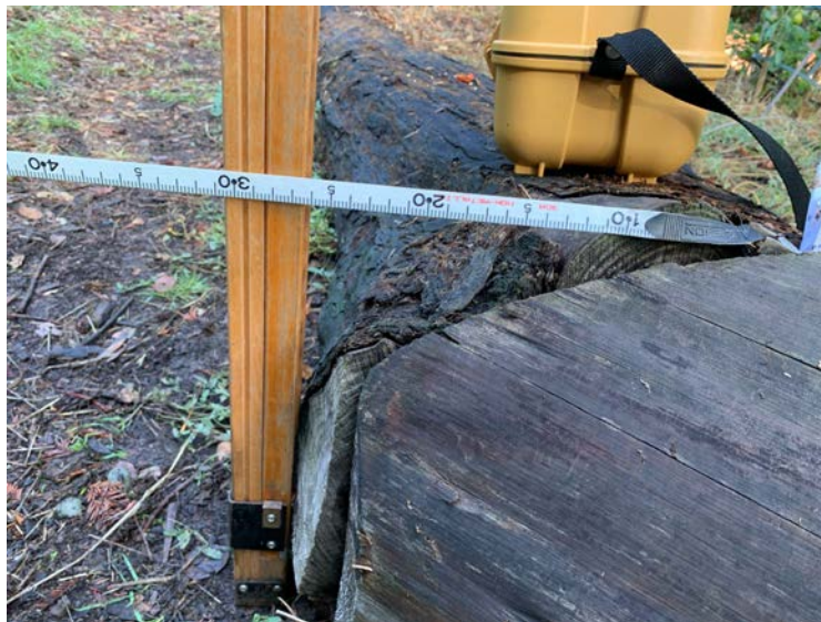
Photo 10. T3 survey starting point. 2022 T3 measurements began at the rod location shown. Measurements taken in the past began at the rebar (not shown) to the right of the log intersection.
