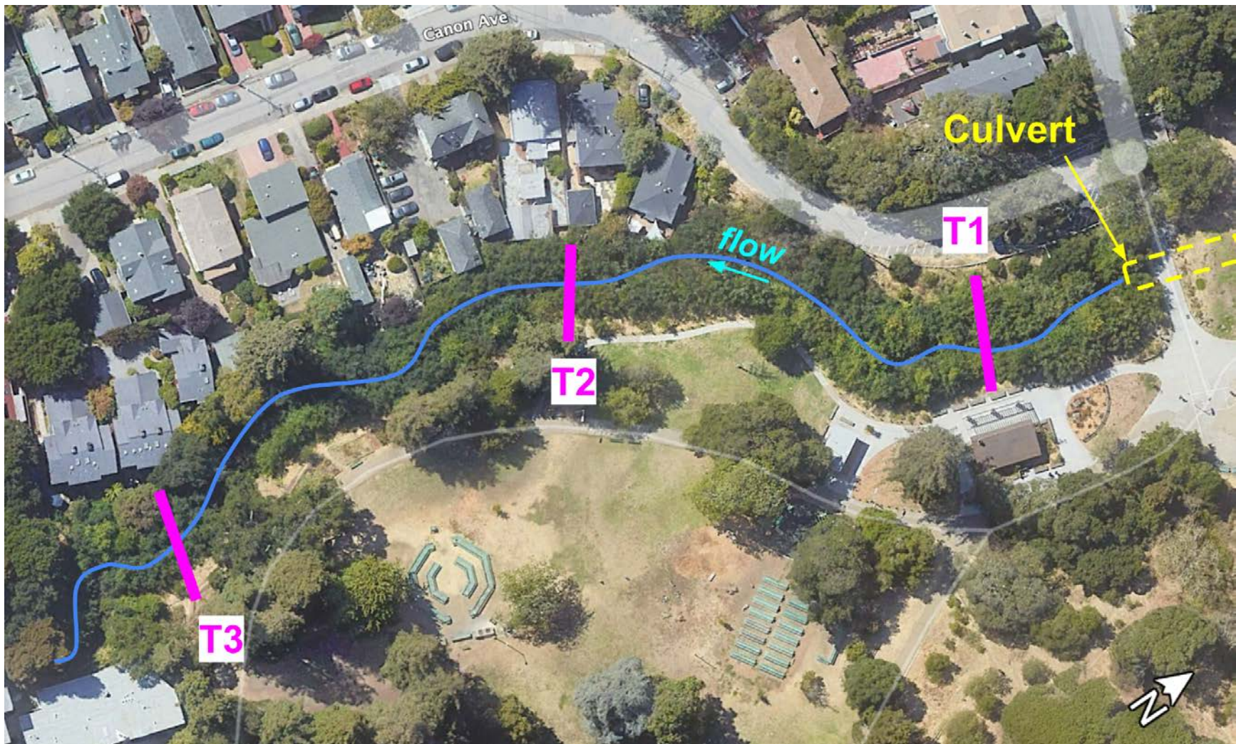
Map 2. Site map depicting the 2016 restoration project reach at Dimond Park (Refer to the black square in Map 1 ). The magenta lines indicate the transects (T1, T2, T3) initially defined by RDG and used for our vegetation and cross-section surveys. The yellow dashed box outlines an existing culvert that feeds the project reach.
