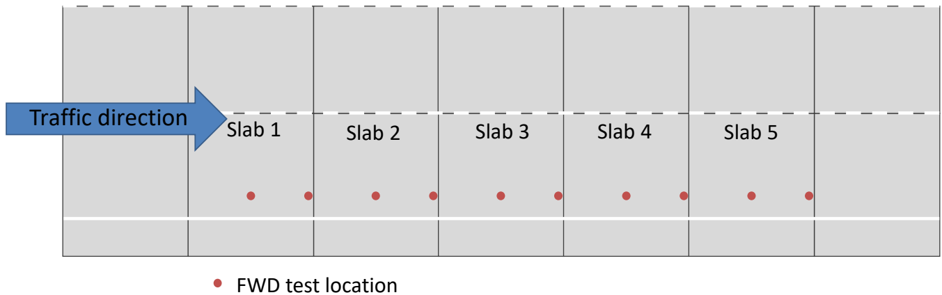
Figure 3.11: Layout of one set of slabs (five consecutive slabs) for FWD testing.
