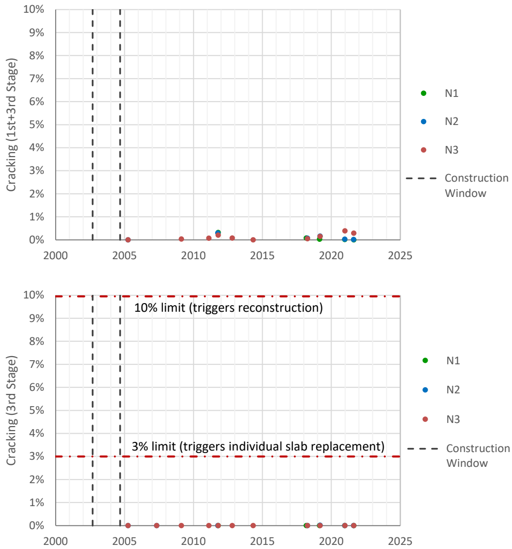
Figure 2.3: Measured first-stage (top) and third-stage (bottom) cracking, I-15-Baker.
