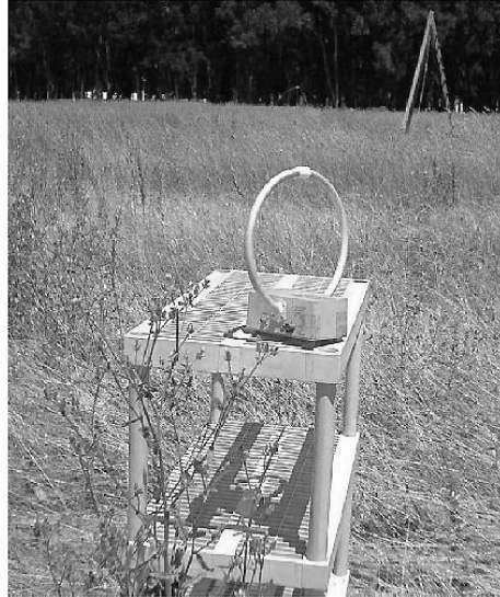
Figure 13. HFI system components. (A) loop magnetic sensor, and (B) stub electric field antenna.
