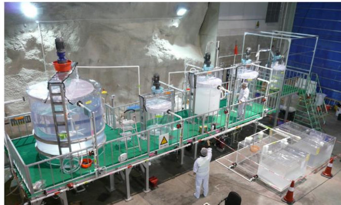
Figure1 (a) three-dimensional diagram (south to north) and (b) photograph of the operation of the production system for liquid scintillators (north to south).
