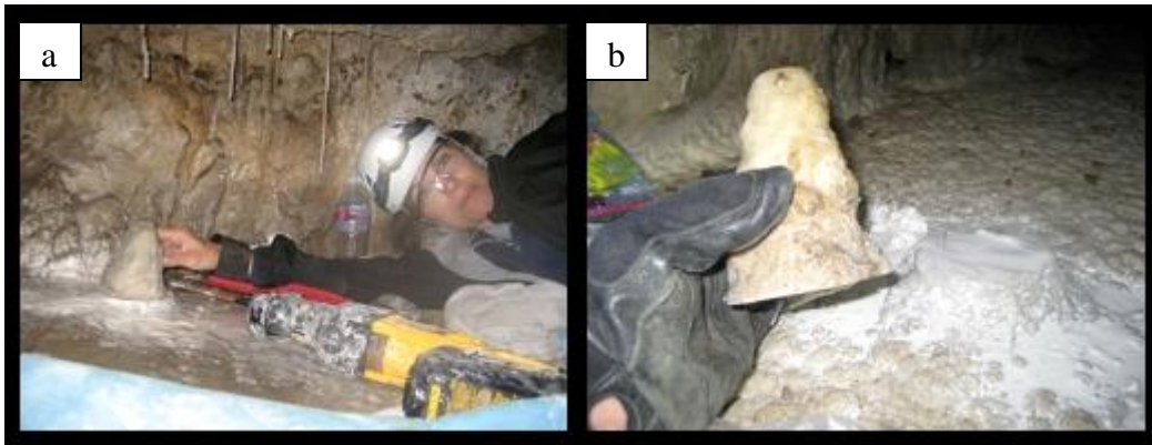
Figure 2.5 Stalagmite collections a) Staryl McCabe-Glynn pouring water continuously over saw blade during stalagmite collection, and b) the stalagmite sample, CRC-3.
