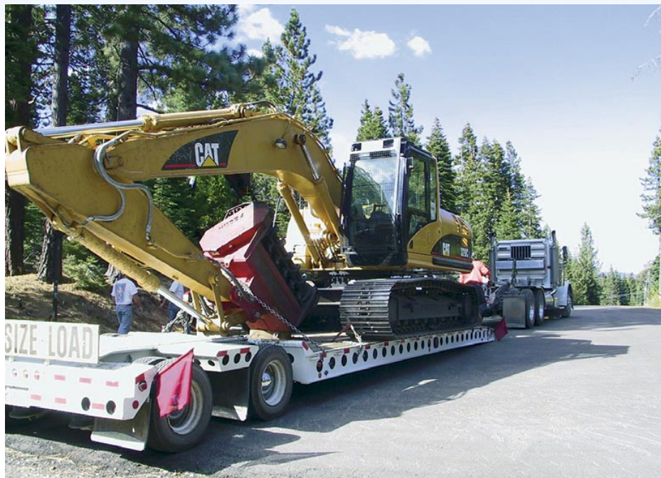
Mechanical mastication is a promising method for thinning overstocked forests. Above, a Fecon Bull Hog BH 80 masticator head is mounted to the boom of a Caterpillar 235 excavator.
