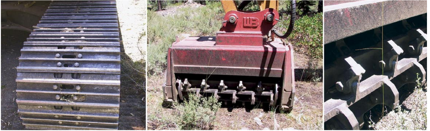
Right and center, the masticator grinds overstocked forest understory and leaves a layer of protective mulch. The authors evaluated whether the large machine's tread, left, contributes to soil compaction and subsequent runoff.
