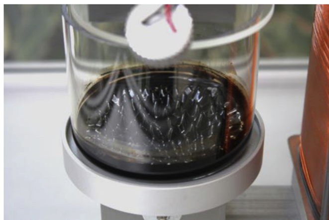
Fig. 7. Response of the ferrofluid to an external magnetic field.
