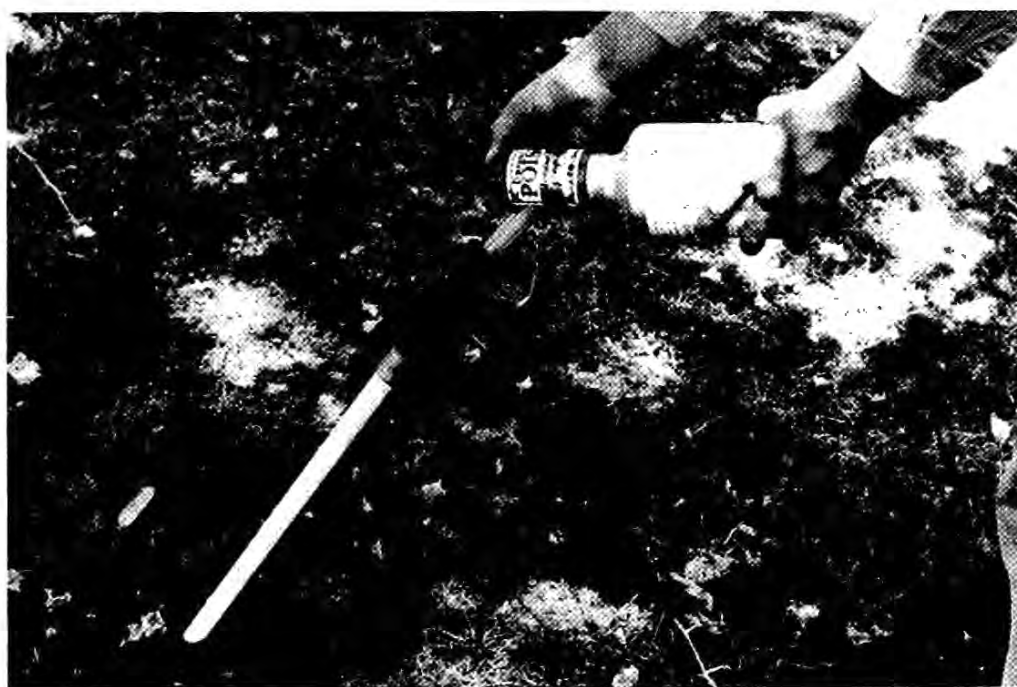
Figure 5. The Degesch mechanical aluminum phosphide pellet applicator.
