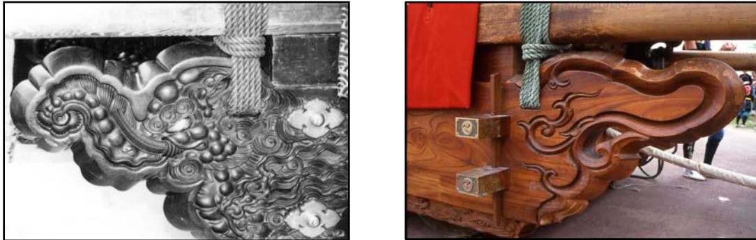
Figure 6. Kibana of Seiryūsha (left) and Miyamotoguruma (right). Note nail covers on left and protruding tenons on right. Source: Author photos.
