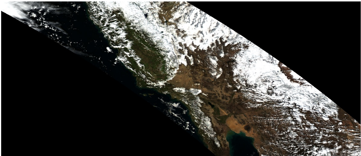
Figure 10. MODIS Aqua, January 23, 2010. Tile H08,V05, true color. Brightness alone might appear to be sufficient to separate clouds and snow from unobscured surface. In fact, many desert soils and urban areas are brighter than many snowy forests and darker clouds.
