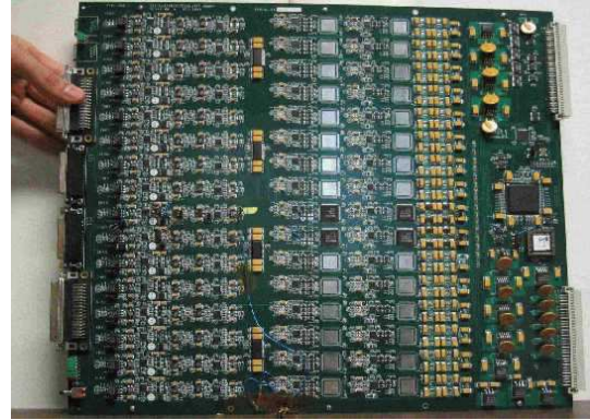
Figure 7. The 16-channel oscillator/demodulator boards provide the AC bias sine-wave carriers which are sent to the bolometers. The carriers with associated sky-signal amplitude modulation are received from the bolometers and SQUID amplifiers, mixed down to base band, and digitized on-board. One oscillator/demodulator channel is required per bolometer, therefore, 60 boards in three 9U VME crates are needed for the SPT receiver.
