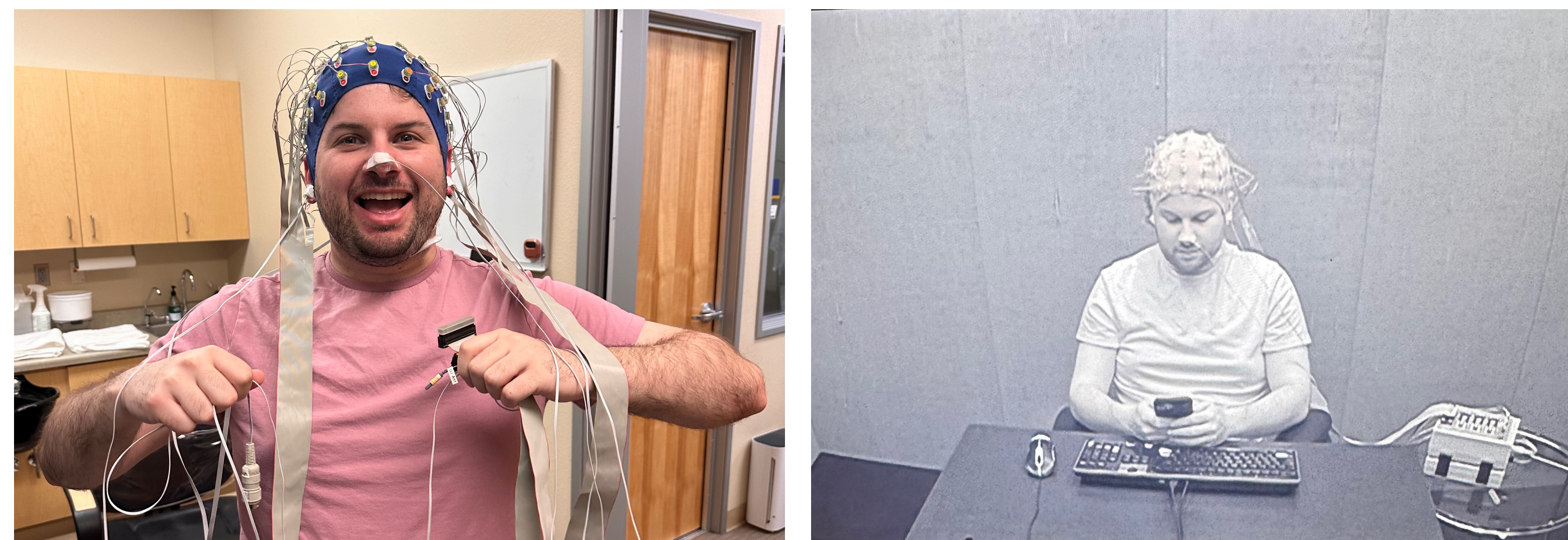
Figure 3. An example of recording EEG auditory and visually-evoked potentials using 64 scalp electrodes and multiple external reference electrodes. These signals are recorded by an acquisition system which tightly links stimulus presentation with evoked potential responses.
