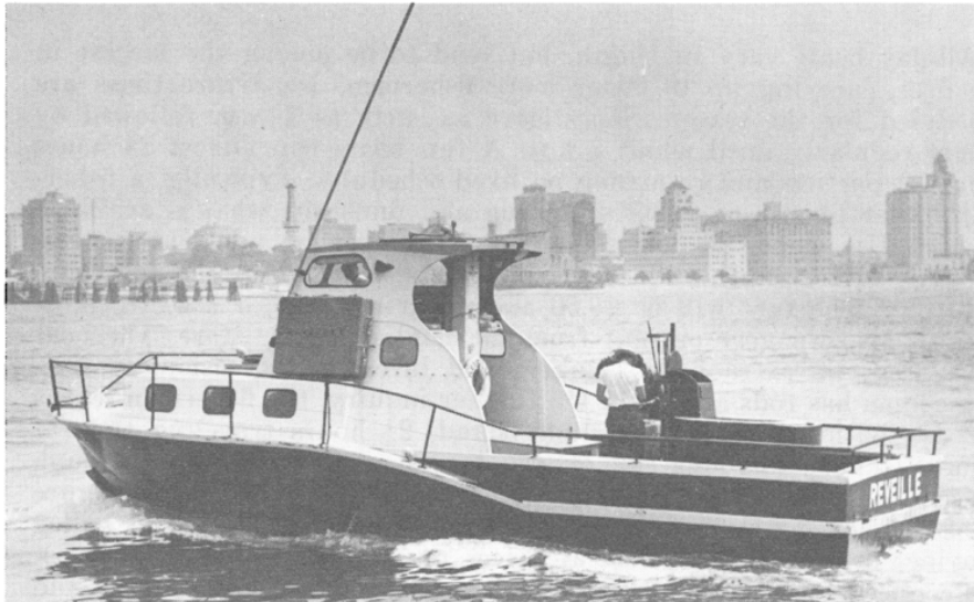
FIGURE 4. A charter-boat about 44 feet long, fishing 20 persons with bunks for 10. Charter boats are predominately owned by individuals and may or may not fish every day during the main season. A boat of this capacity charters for about $200.
