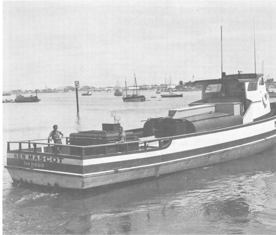
FIGURE 2. An all-day party boat of late design, about 65 feet long, carrying 60 passengers. About 30 boats of this type have been launched in recent years. Most are powered with twin-engine diesels. Photograph courtesy H. & M. Sportfishers Inc., San Diego.
